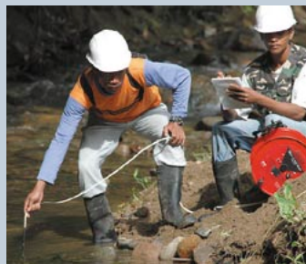
Above: Field Technicians, Ronnie and Doming Puli, conducting water level monitoring along the Lawit River near the Tampakan deposit.
